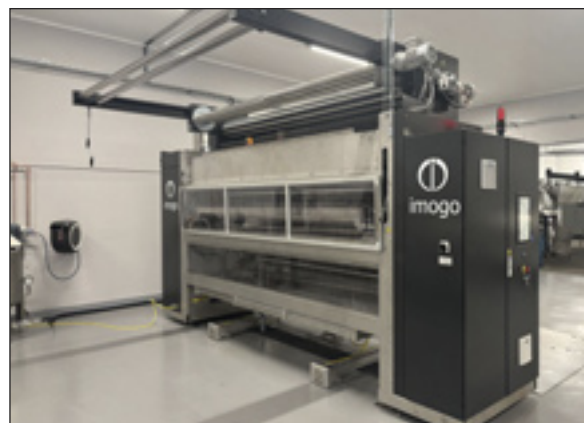
The Dye-Max application unit can spray-dye up to 1.5 t of fabric a day.
