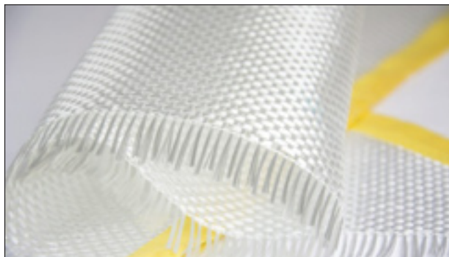
Woven glass-fibre fabrics such as this are used to manufacture composite copper-clad laminates.
