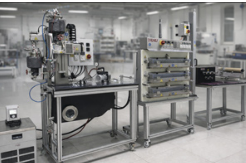
A wet-spinning line from Dienes Apparatebau GmbH. The company will tell visitors to its stand that in order to develop new fibres, filaments and yarns, companies need efficient, modular, flexible and, in part, self-optimising experimental working systems such as this that can gather data on the process being carried-out.
