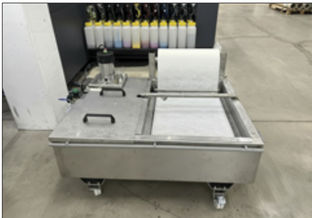
Zimmer Austria's Colaris-TeX digital printer can be equipped with a water-treatment module to minimise the amount of wastewater it creates.
