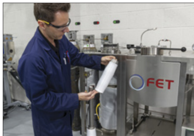
Fibre Extrusion Technology (FET) has developed technology that enables it to use supercritical carbon dioxide as a solvent for the production of ultra-high molecular-weight polyethylene fibres. Here, FET's Senior Material and Process Scientist, Kris Kortsen, inspects a batch of fibres.
