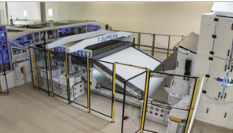
A T-Suprema production line for needlepunched nonwovens, developed by Trützschler Nonwovens in partnership with Texnology Srl (see also, page 11).
