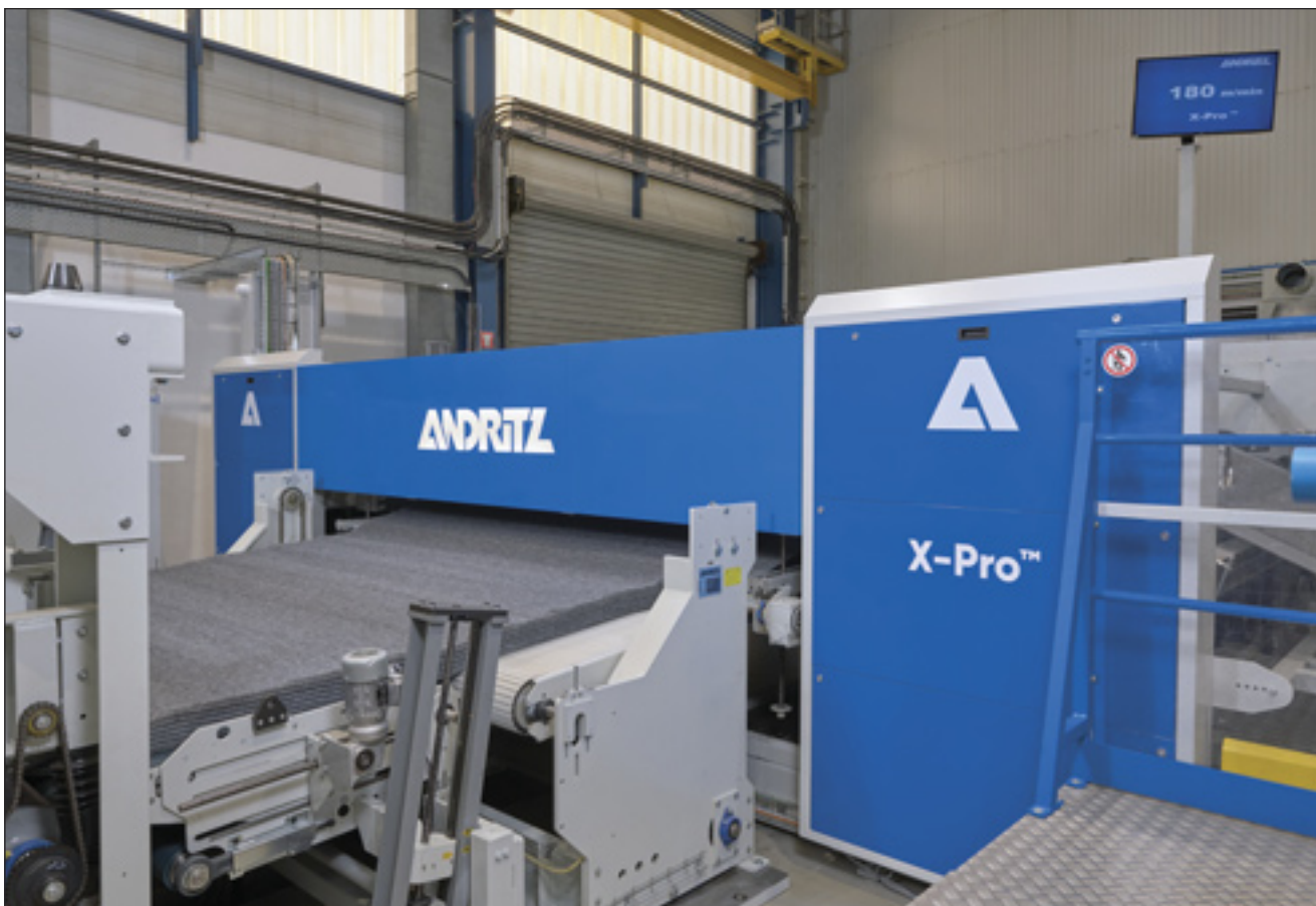
At Techtextil , Andritz will introduce its X-Pro crosslapper for use with needlepunch and hydroentanglement lines.
