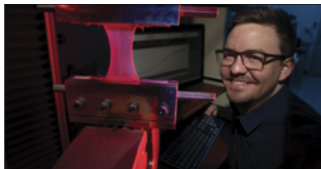
Lincoln-Laboratory staff-member Steve Gillmer tests the elasticity of a bioabsorbable fabric in order to compare its stiffness to those of different types of human tissue.
