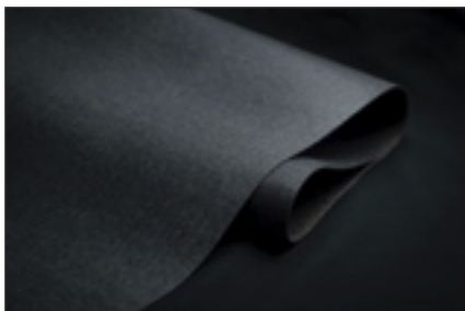
Lastan is a flame-resistant fabric made by air-baking an acrylic fibre at 200–300°C and is characterised by high flame-retardance and low electrical conductivity.
