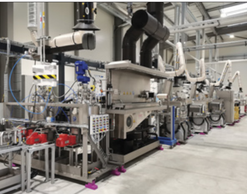
A wet-spinning line from Dienes Apparatebau GmbH of Mühlheim am Main, Germany. The company will tell visitors to its stand that in order to develop new fibres, filaments and yarns, companies need efficient, modular, flexible and, in part, self-optimising experimental working systems that can gather data on the process being carried-out.
