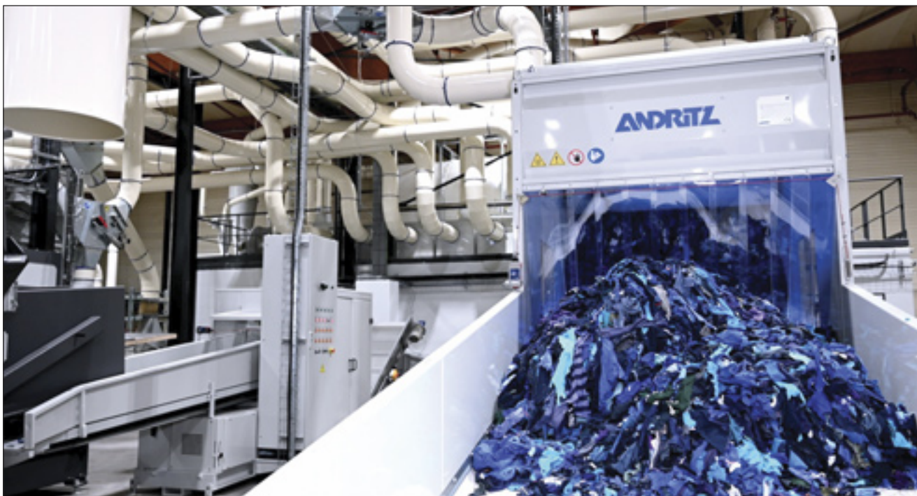
Sorted and cut textile waste ready for tearing at Nouvelles Fibres Textiles' facility in Amplepuis, France.
