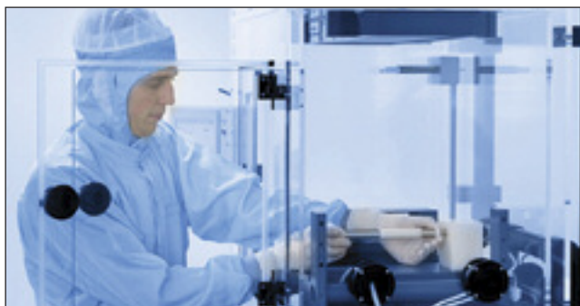
IME Medical Electrospinning has developed an electrospinner that it says can reproducibly and continuously manufacture micro- to nanometre-scale biocompatible fibres.
