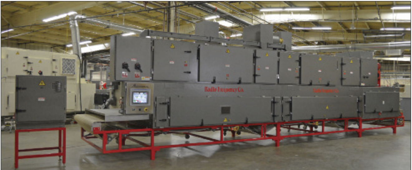
Radio Frequency Co's radio-frequency drying system can heat nonwovens throughout their entire thickness simultaneously.
